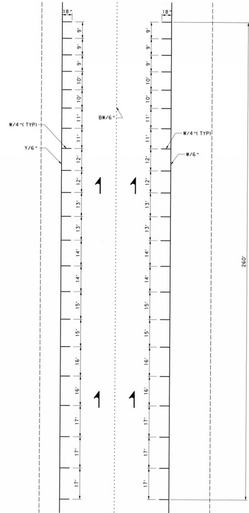
**OPTICAL SPEED BAR DETAIL (45 MPH TO 25 MPH)**
