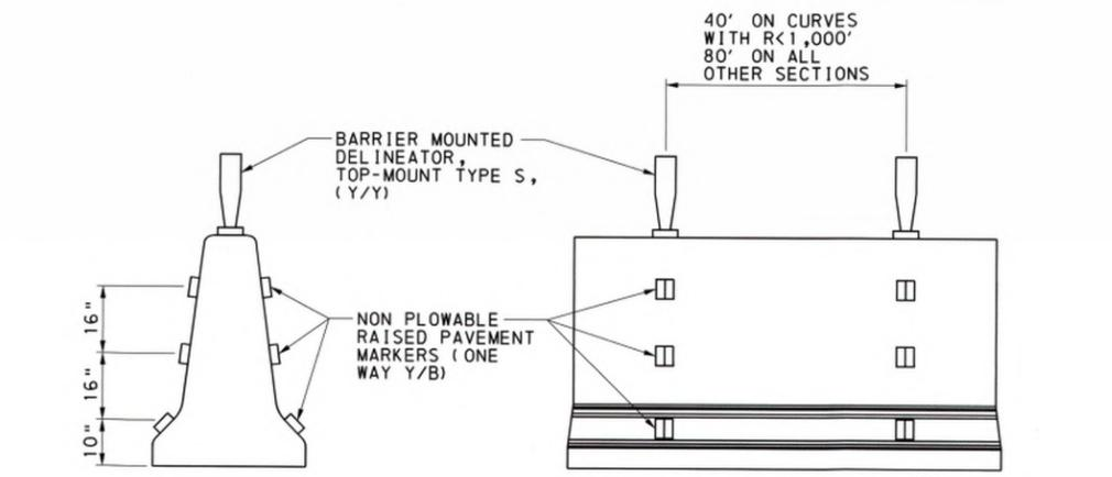
**CONCRETE GLARE SCREEN MEDIAN BARRIER DELINEATION DETAIL**
